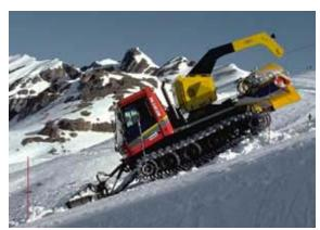
Before the first pole the snowcat has to start pushing up the snow to make a pile at the pole.
