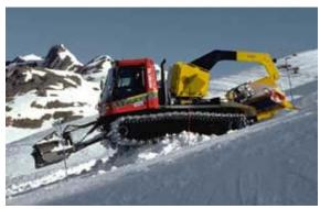
Before the cat dives over the edge of the snowpile it is very important, that the blade stays lifted up. While diving over the edge of the snowpile the cat should be held by the winch so it doesn't slide
