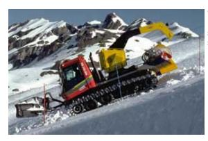
When the snowpile is at the right location the cat has to lift the blade and should carefully drive on top of the snowpile.
