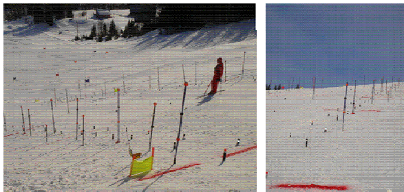
Figure 1. Experimental set-up indicating control points, non-control points, camera positions, and gate positions. The global reference system is also indicated.
