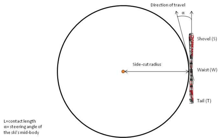
Figure 2.1: The side-cut radius and the steering angle of a modern slalom ski.
