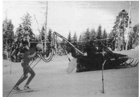
Fig. 1. Collection of expiratory air from snow-scooter during uphill skiing at race speed using the classical technique
